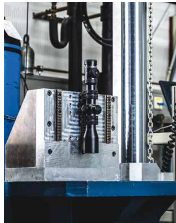
Simulation of extreme situations: extreme temperature variations within minutes and shot simulations at 1,500 times the force of gravity.
