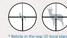
* Reticle in the rear (2) focal plane
