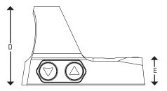
A – 2.1 in / 54mm B – 1.3 in / 32mm C – 1.1 in / 28mm D – 1.4 in / 35mm E – 0.5 in / 12mm
